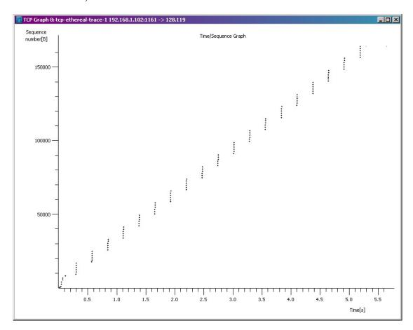
Here, each dot represents a TCP segment sent, plotting the sequence number of the segment versus the time at which it was sent. Note that a set of dots stacked above each other represents a series of packets that were sent back-to-back by the sender. Answer the following questions for the TCP segments the packet trace *tcp-ethereal-trace-1* in <a href="http://gaia.cs.umass.edu/wireshark-labs/wireshark-traces.zip">http://gaia.cs.umass.edu/wireshark-labs/wireshark-traces.zip</a>
