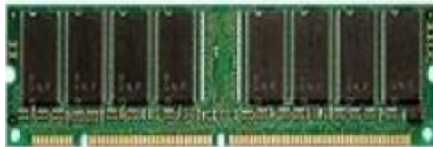
168 pin SDRAM DIMM
