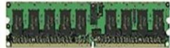
240 pin DDR-2 DIMM
