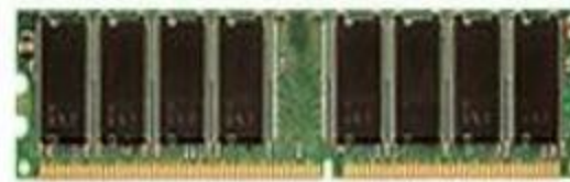
184 pin DDR DIMM
