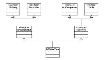
Figure 5. Example of two role models combined in a single component.
