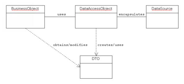
The following sequence diagram shows the interaction among the participants in the Data Access Object pattern. The BusinessObject creates the DataAccessObject and uses it to get data. The DataAccessObject encapsulates access to a DataSource. The Data Access Object also manages creation of and updates to data in the DataSource. A Data Access Object consists of getter and setter methods to manipulate the data.
