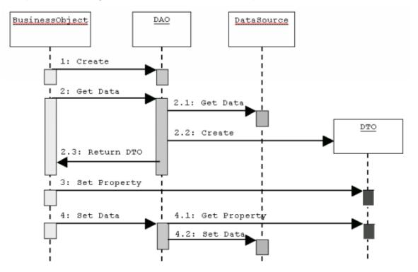
As you can see, the DAO is responsible for creating Data Transfer Objects (DTOs), which are convenient means to pass data between BusinessObjects and DAOs. Once the BusinessObject completes processing of the DTO, it can return the DTO to the DAO. The DAO can write the changes out to the DataSource to complete the transaction.
