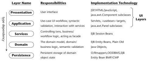
Figure 6.4 The layering in a J2EE system.
