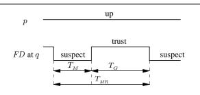
Figure 4. Mistake duration  $T_M$ , good period duration  $T_G$ , and mistake recurrence time  $T_{MR}$
